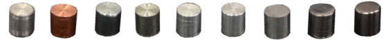
Figure 1 – Specimens for uniaxial compression with initial diameter \phi_0 = 6 \text{ mm} and initial height h_0 = 6,4 \text{ mm} . From left to right: (i) pure Aluminium, (ii) pure Copper, (iii) pure Zinc, (iv) pure Tin, (v) AA1085, (vi) AA1050, (vii) AS7G03+05U, (viii) AISI1045 and (ix) Ti6Al4V.
